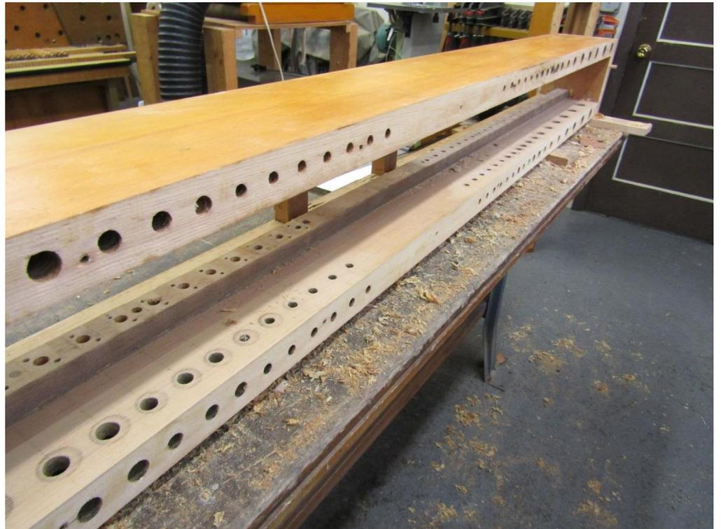
New leather gasketing was applied to the perimeters of the windchest frames, punched to permit transmission of both pneumatic signals and speaking wind pressure to the pipes above. Most importantly, a new (red) rubbercloth membrane was applied to the tops of the Ventil boxes, glued around the wind holes, as a certain preventative of spurious leakage and ciphers, in the long term.
