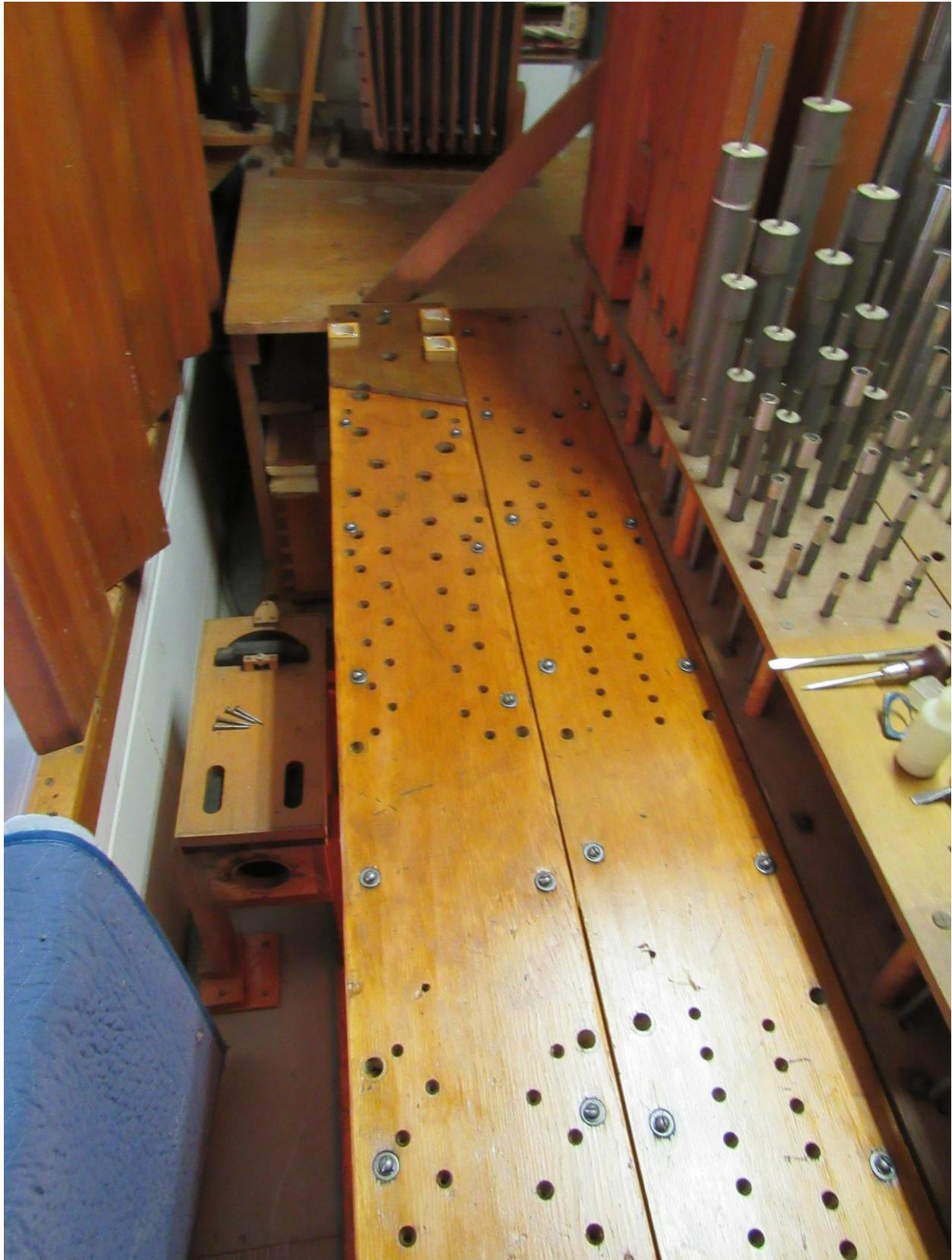
Photo-documentation at the completion of work in September 2019 - restoration of two unit stops, Open Diapason and Voix Celeste ranks, at the front of the main windchest in the organ chamber. You can compare this view to that shown in the very first image at the start of this presentation... almost exactly the same shot, but certainly a “before-and-after” scenario, with clear improvements.
