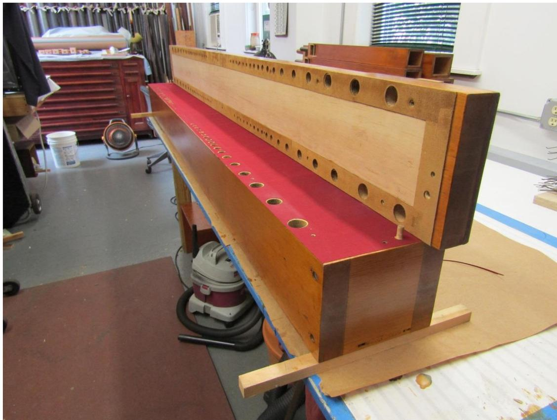
The interior **Note-Action Motors** suffered also from the water intrusion; each of these units was dismantled, tested under pressure, releathered as necessary, and ultimately remounted securely inside the respective Ventil boxes. However, every single action motor received a fresh leather mounting gasket and a new valve face. As initially dismantled, and during testing, these pneumatic actions looked like this:
