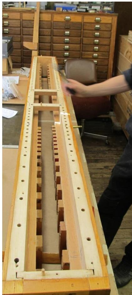
The **Bottom-boards** of the Ventil boxes had to be treated delicately because of the aged, proprietary magnets and their light-gauge wiring, but yet to clean thoroughly the ports, seats, and armatures for reliable playing responsiveness. The process began by lifting the magnets and armatures from their seats in the bottom-boards:
